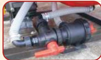
Inspected suction filter with valve and a connection for the tank filling hose and a 3-ways ball valve.
